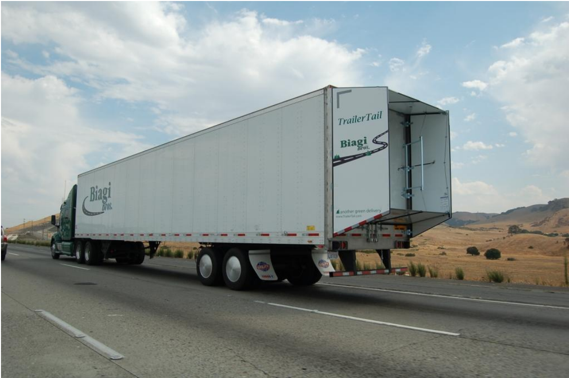
California trailer equipped with ATDynamics TrailerTail®, aerodynamic rear fairing
